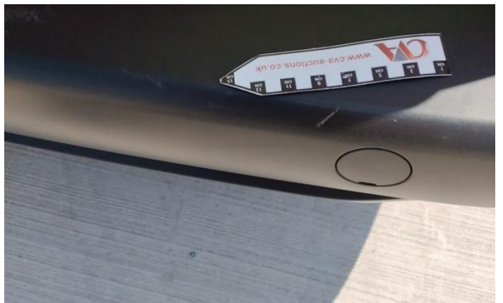
4: Qtr Panel nsr Scratched UpTo 25mm Thru Paint
