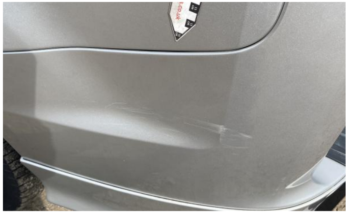
4: Door osf Dented With Paint Damage
