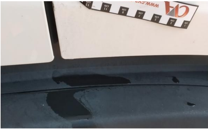
9: Wing Front Arch Extension ns Broken Replace
