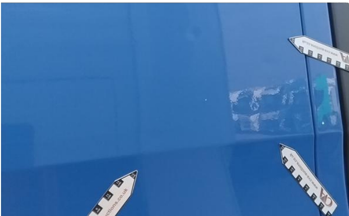
5: Panel Front Scratched Over 25mm Thru Paint
