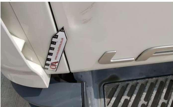
5: Wing nsf Cracked Replace
