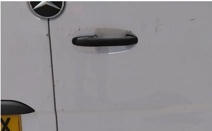
15: Door nsr Scratched UpTo 25mm Thru Paint
