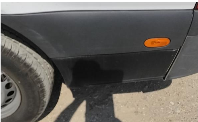
11: Qtr Panel nsr Dented Over 30mm
