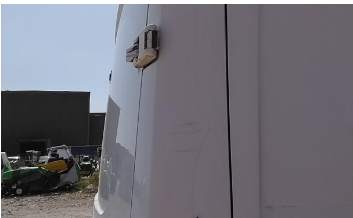
17: Door osr Scratched Over 25mm Thru Paint
