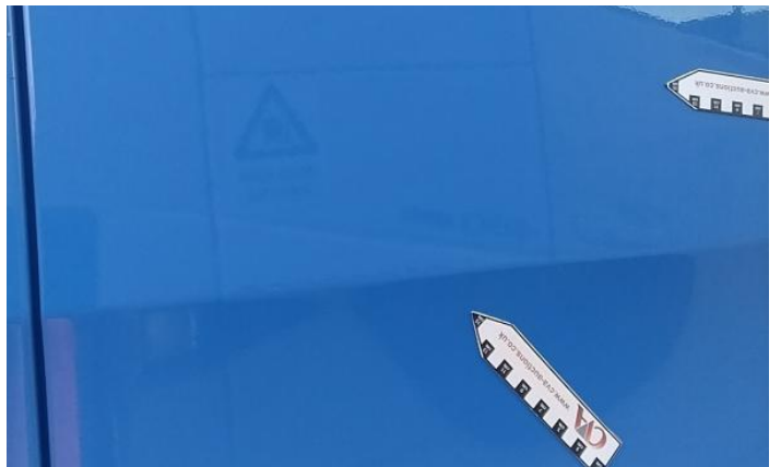
6: Wing nsf Scratched Over 25mm Thru Paint
