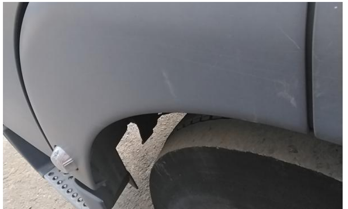
4: Door nsf Scratched Over 25mm Thru Paint
