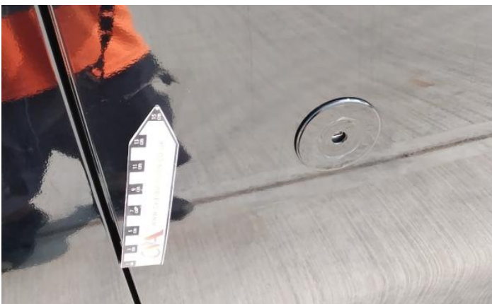
5: Bumper Rear Scratched 25 to 100mm Thru Paint
