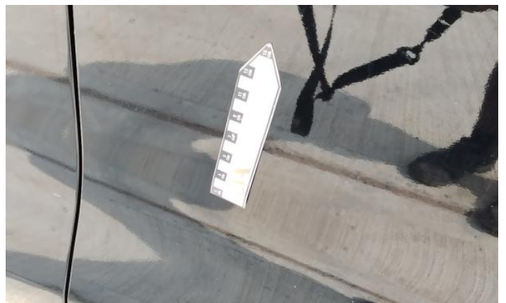
6: Bumper Rear Scratched 25 to 100mm Thru Paint
