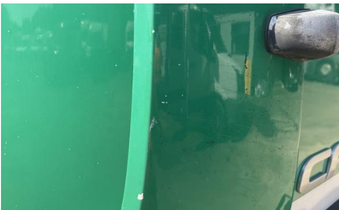
5: Door osf Dented Over 30mm
