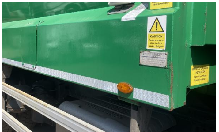
4: Wing osf Scratched Over 25mm Thru Paint
