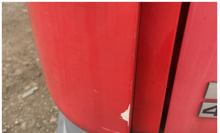
10: Door nsf Dented With Paint Damage
