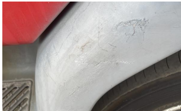
9: Qtr Panel nsr Rusted Over 5mm
