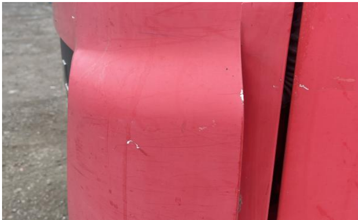
9: Qtr Panel nsf Rusted Over 5mm
