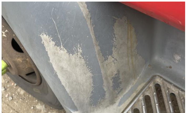
4: Wing osf Cracked Replace
