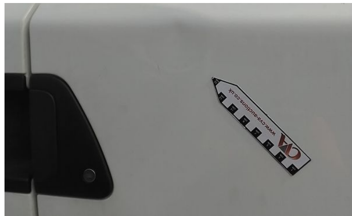
3: Door nsf Dented Over 30mm
