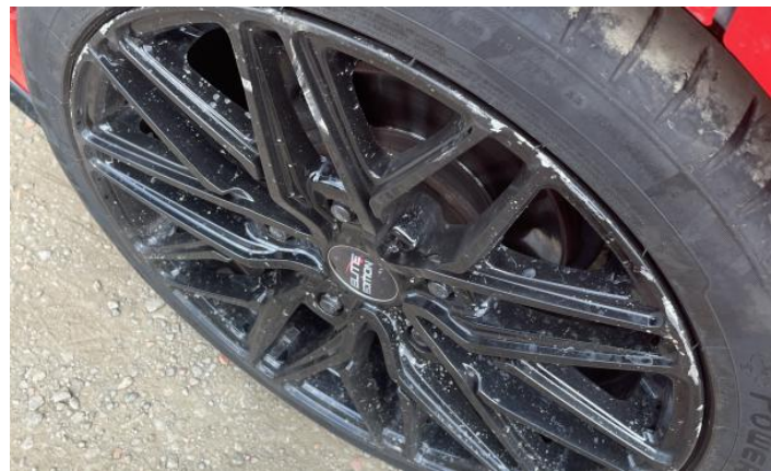
9: Wheel nsf Dented Over 30mm (Alloy)
