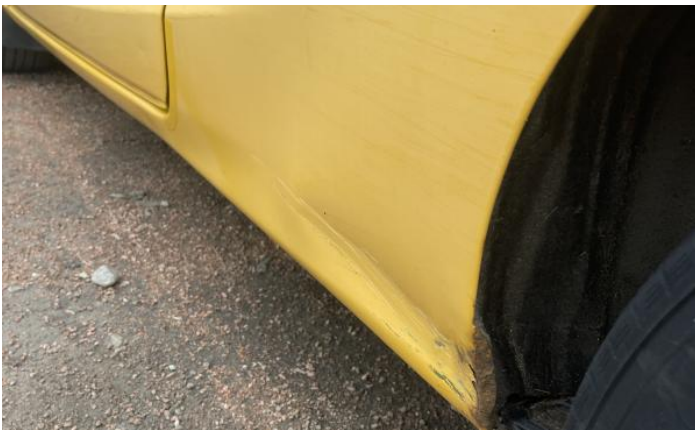
5: Qtr Panel osr Dented With Paint Damage
