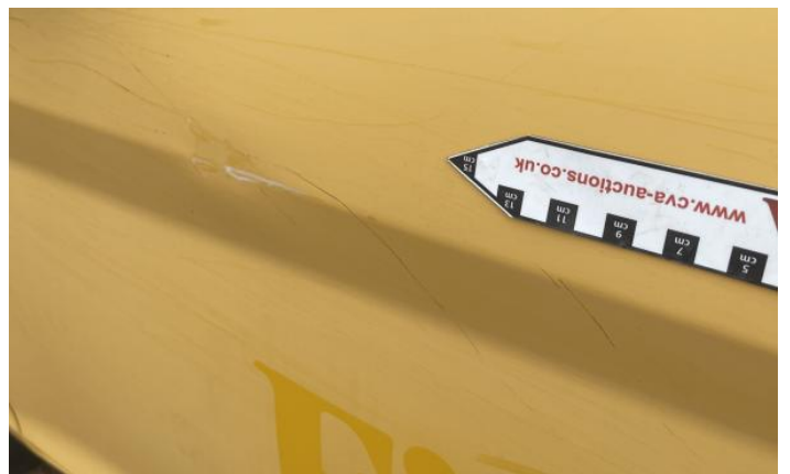
6: Bumper Rear Scratched Over 100mm Thru Paint
