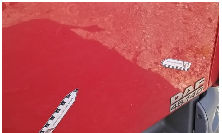
6: Qtr Panel nsr Scratched Over 25mm Thru Paint
