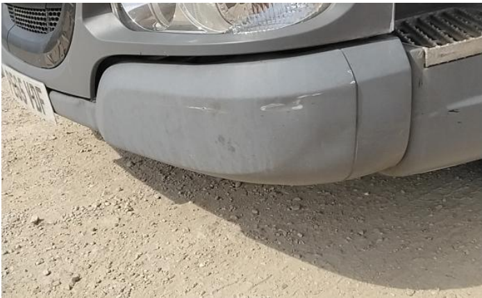
3: Bumper Front Chipped Multiple Chips
