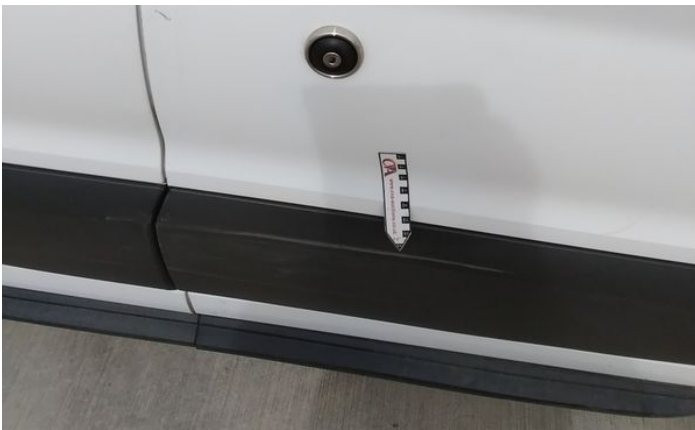
29: Qtr Panel Moulding os Scratched (Painted) Over 25mm Thru Paint
