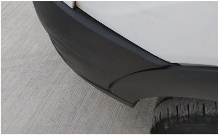
3: Bumper Front Scratched Over 100mm Thru Paint
