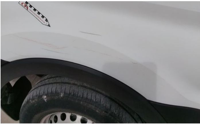
21: Door osr Scratched Over 25mm Thru Paint
