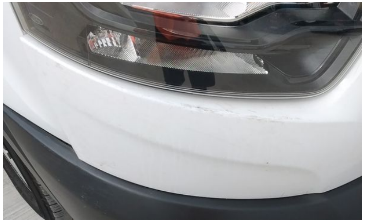
34: Wing Front Arch Extension os Broken Replace
