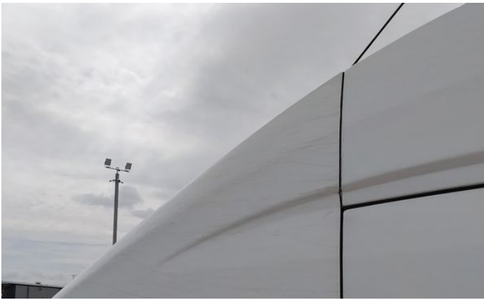
9: Door nsf Scratched Over 25mm Thru Paint
