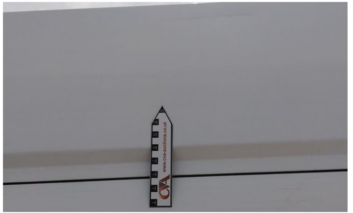
16: Qtr Panel nsr Scratched Over 25mm Not Thru Paint
