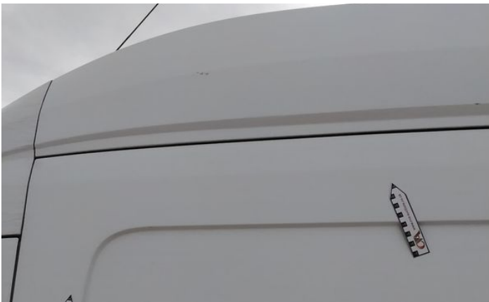
11: Roof Scratched Over 25mm Thru Paint
