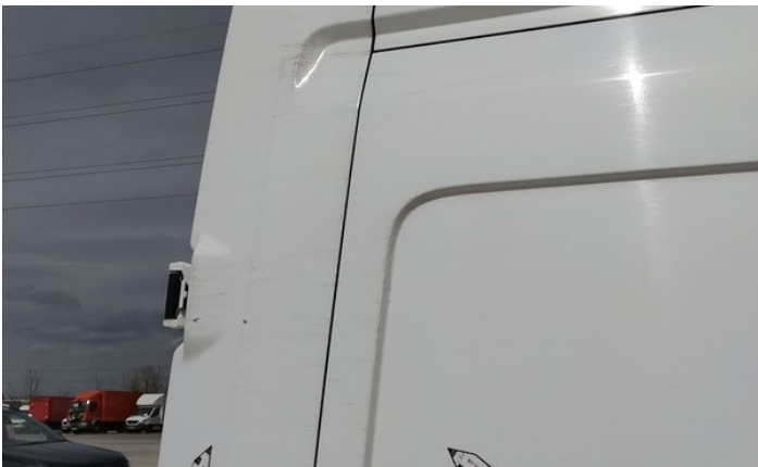
23: Qtr Panel osr Scratched Over 25mm Thru Paint
