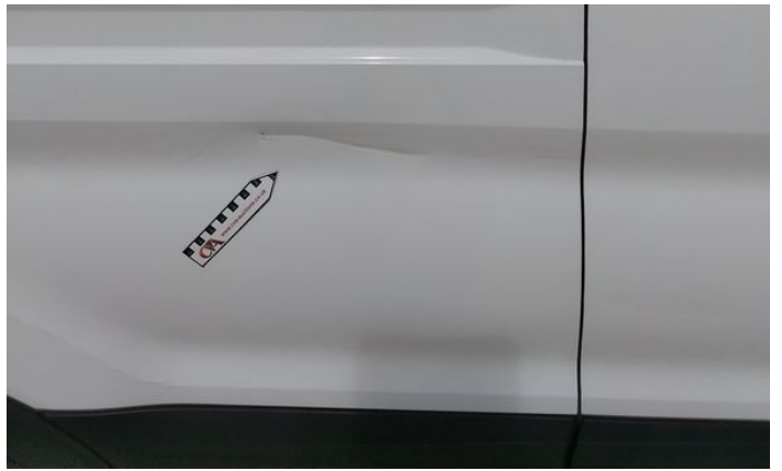
22: Qtr Panel osr Scratched Over 25mm Thru Paint
