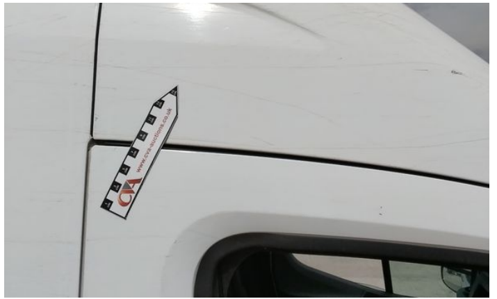
28: Qtr Panel Moulding os Scratched (Painted) Over 25mm Thru Paint
