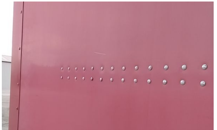
6: Wing nsf Scratched Over 25mm Thru Paint
