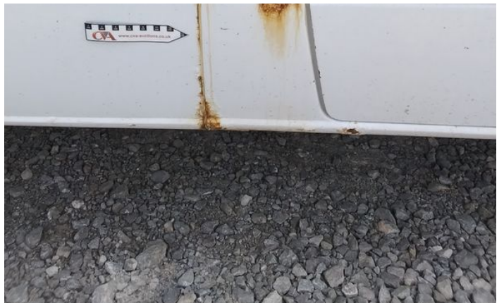
18: Qtr Panel osr Rusted UpTo 5mm
