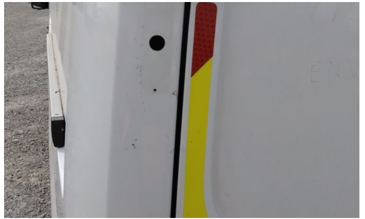
10: Qtr Panel nsr Poor Previous Repair Paint Flake
