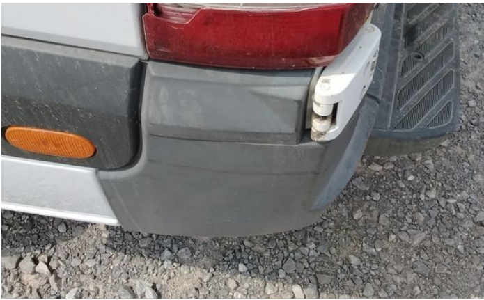
9: Qtr Panel nsr Cracked Replace
