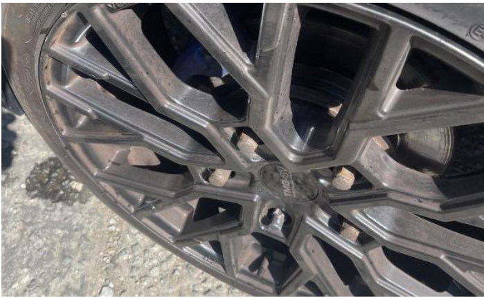
9: Wheel nsr Damaged Replace
