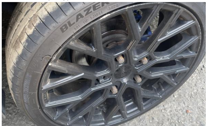
6: Wheel osr Dented Over 30mm (Alloy)
