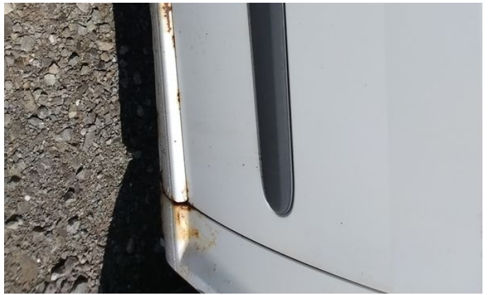
4: Door nsf Rusted Over 5mm
