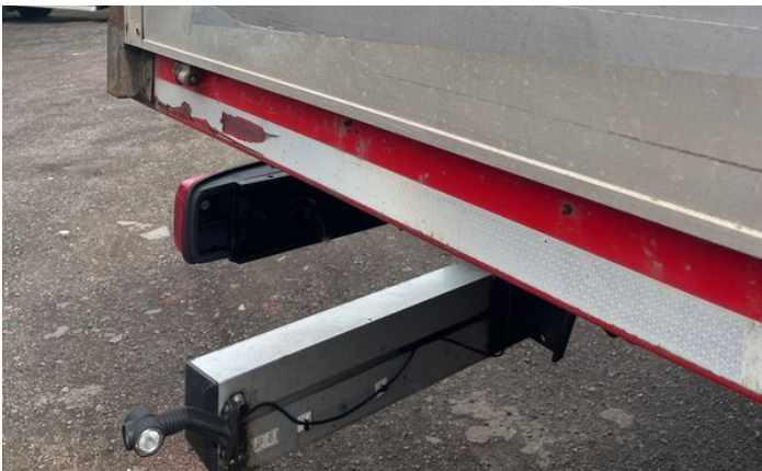
5: Wing osf Scratched Over 25mm Thru Paint
