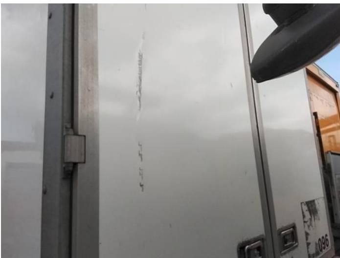
7: Door nsr Dented With Paint Damage
