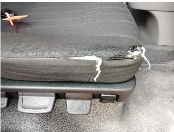
13: Seat Base Cover osf Torn Over 3mm
