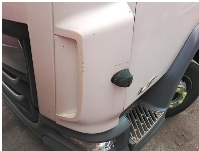
2: Panel Front Scratched Over 25mm Thru Paint
