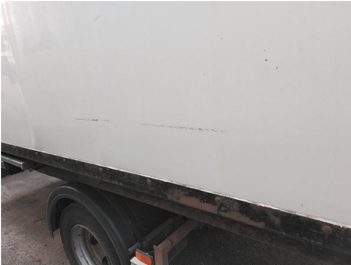
9: Qtr Panel osr Scratched Over 25mm Not Thru Paint
