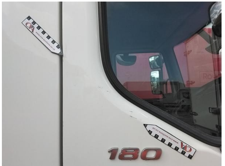
12: Door osf Scratched Over 25mm Thru Paint
