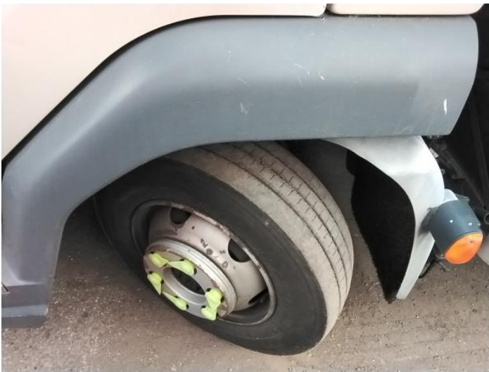
5: Wing nsf Scratched Over 25mm Thru Paint
