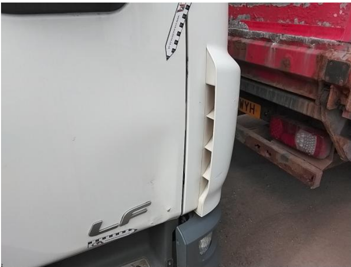
11: Door osf Dented With Paint Damage
