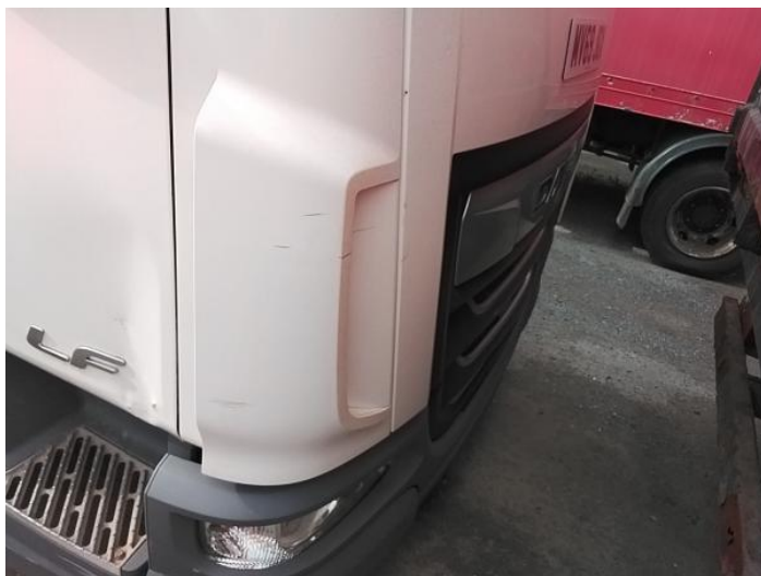
1: Panel Front Scratched Over 25mm Thru Paint
