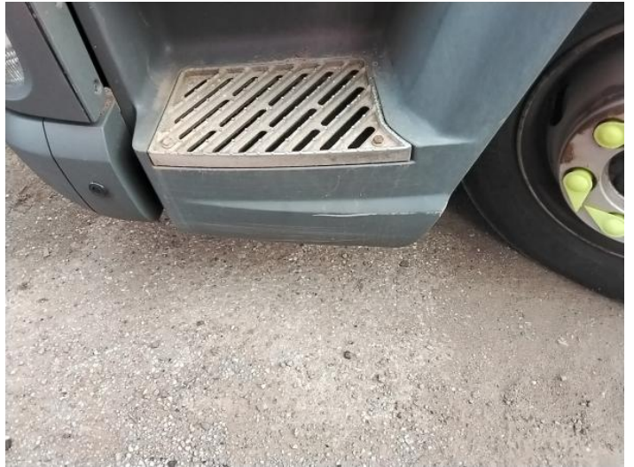
4: Bumper Front Moulding Scuffed (Unpainted) Over 100mm
