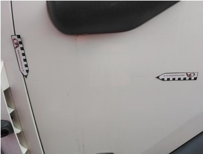
3: Door nsf Scratched Over 25mm Thru Paint
