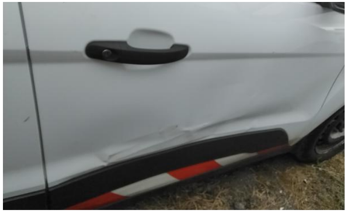
4: Qtr Panel nsr Dented With Paint Damage
