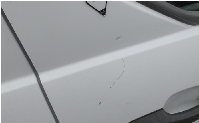
5: Qtr Panel nsr Dented With Paint Damage
