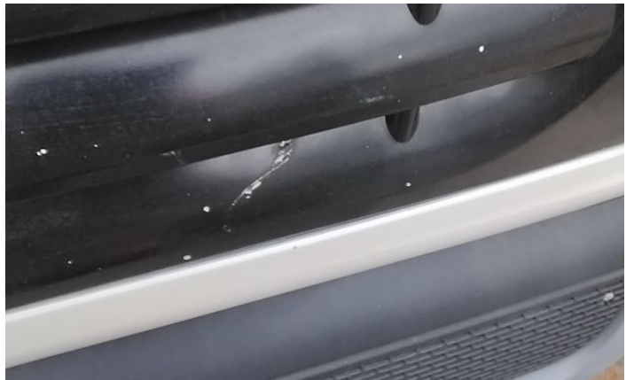
4: Bumper Front Dented With Paint Damage
