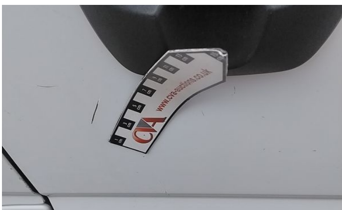
5: Door nsf Scratched Over 25mm Thru Paint
