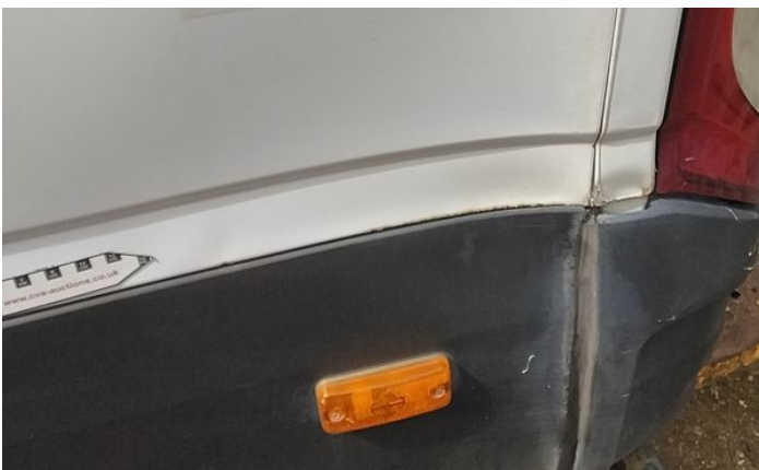
5: Qtr Panel nsr Dented Over 30mm
