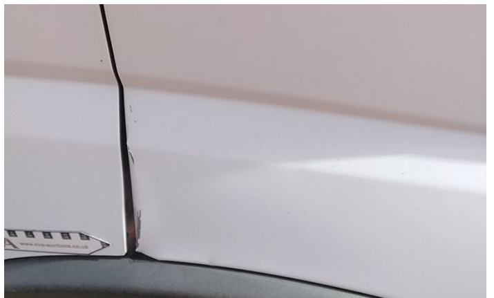
16: Door nsr Dented Over 30mm
