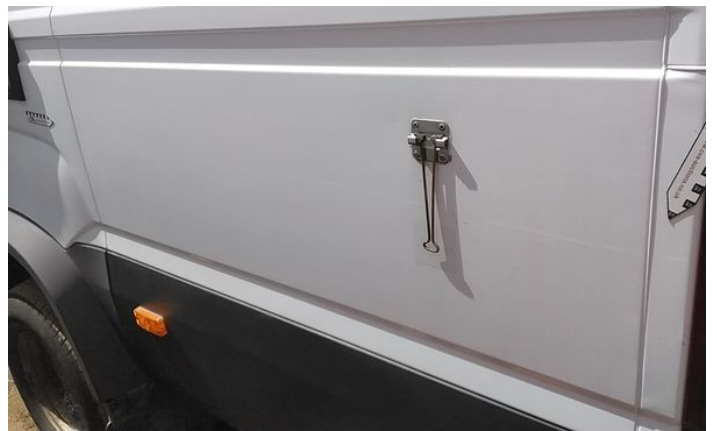
10: Qtr Panel nsr Dented With Paint Damage
