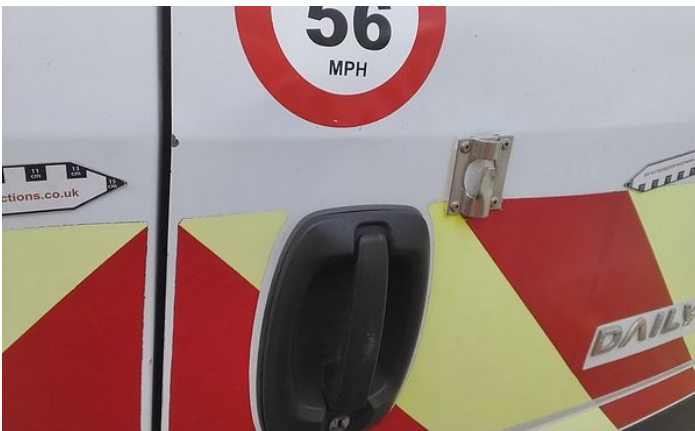
15: Door nsr Dented With Paint Damage
