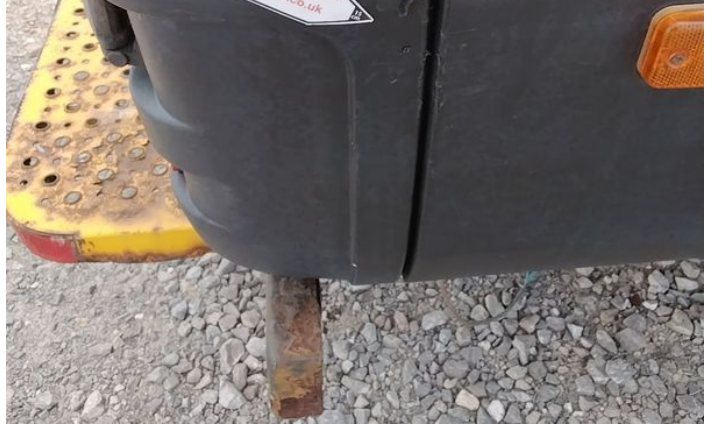
10: Door osr Rusted UpTo 5mm
