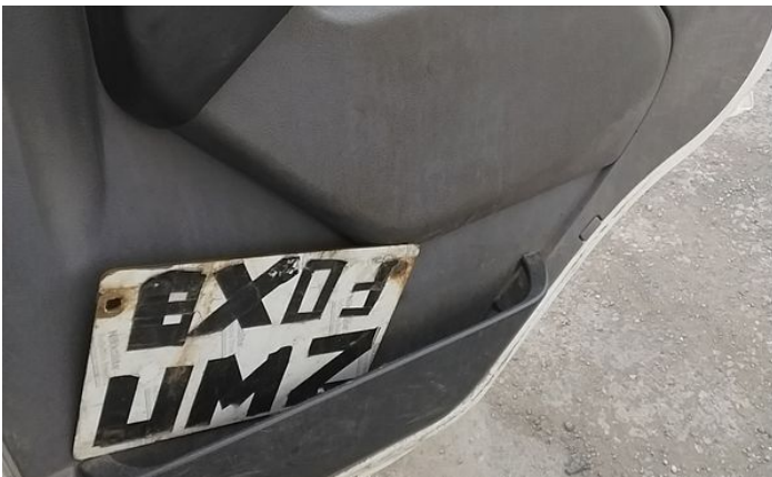
11: Door osf Dented With Paint Damage
