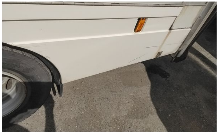
6: Qtr Panel Moulding ns Scratched (Painted) Over 25mm Thru Paint
