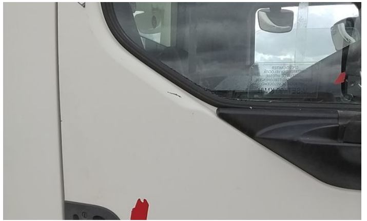
10: Qtr Panel osr Cracked Replace
