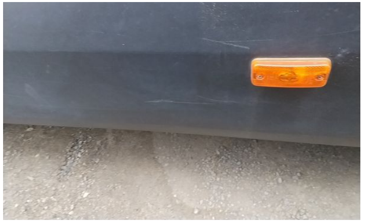
4: Door osf Scratched Over 25mm Thru Paint
