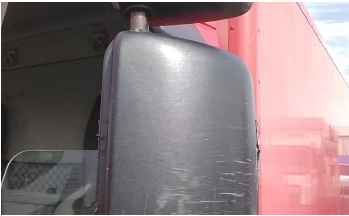
3: Panel Front Scratched Over 25mm Thru Paint
