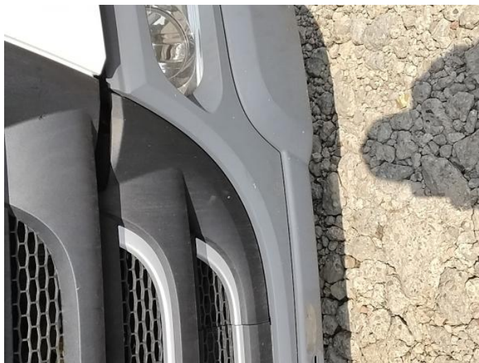
2: Bumper Front Cracked Over 25mm
