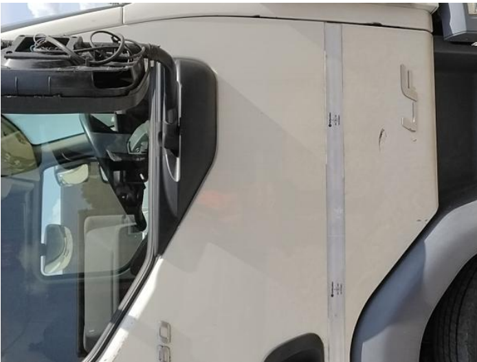
13: Door osf Scratched Over 25mm Thru Paint
