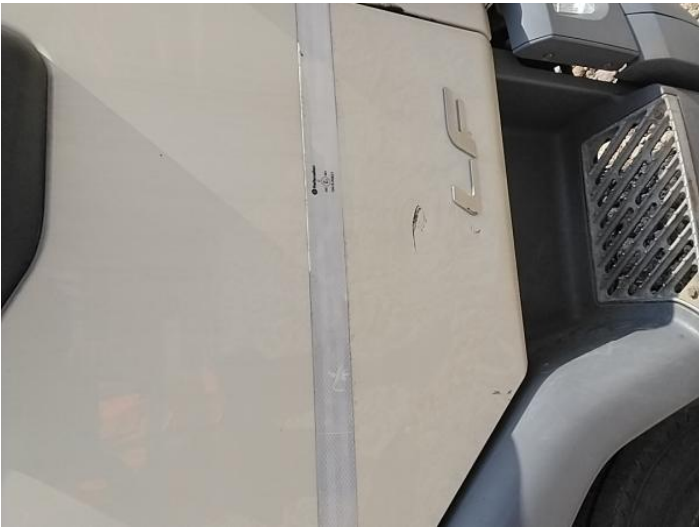
12: Door osf Dented With Paint Damage
