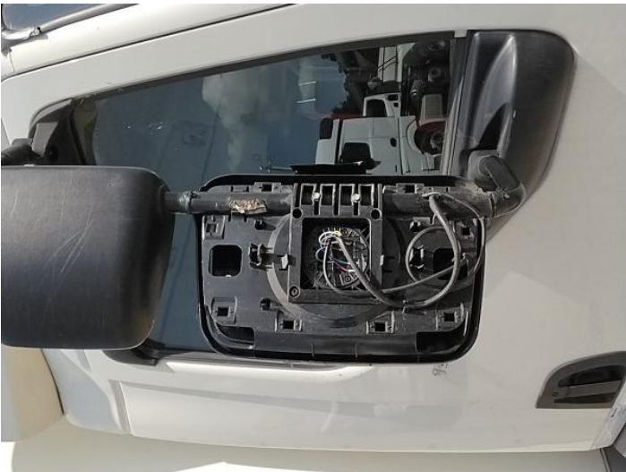
14: Door Mirror Assy osf Missing Replace
