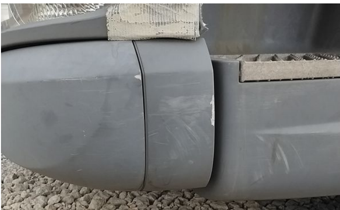
5: Wing nsf Scratched Over 25mm Thru Paint
