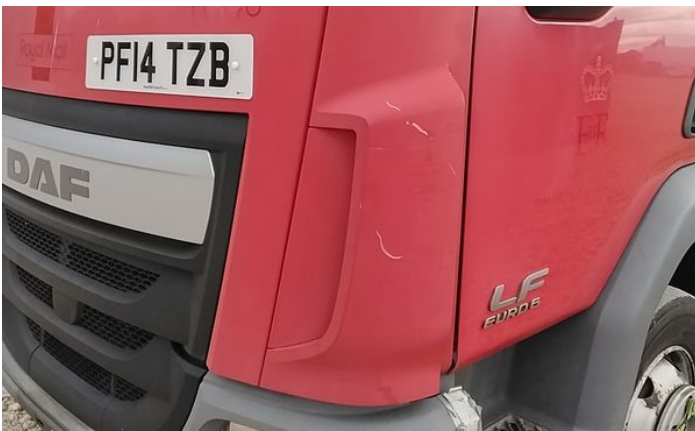
3: Bumper Front Scratched UpTo 25mm Thru Paint
