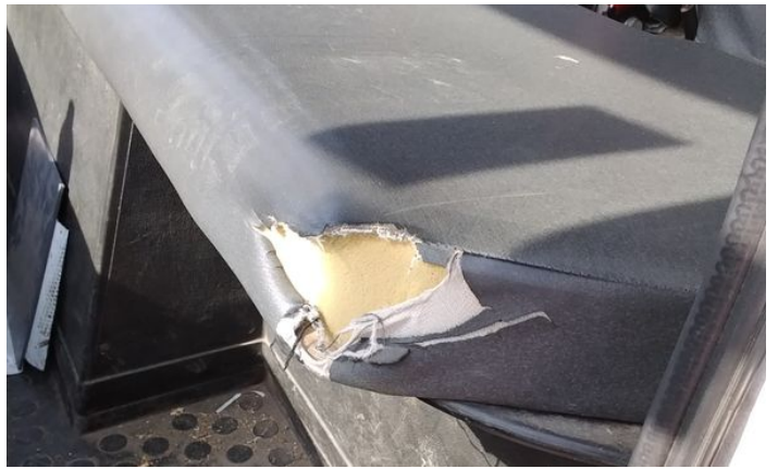
16: Centre Console Front Broken Replace
