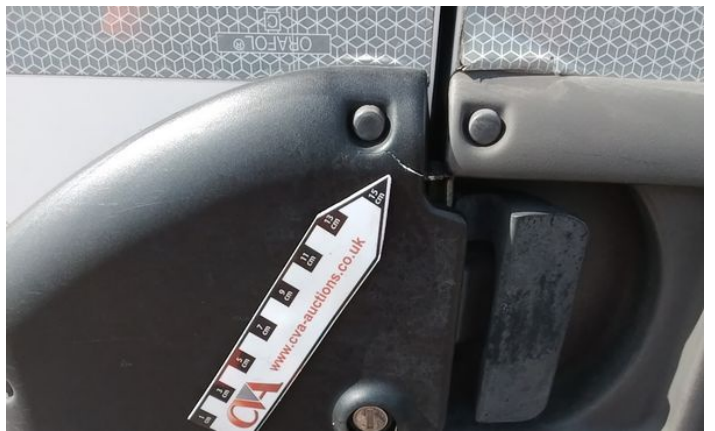
4: Wing nsf Cracked Replace
