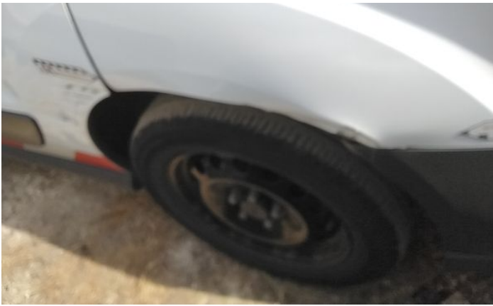
3: Qtr Panel nsr Dented With Paint Damage
