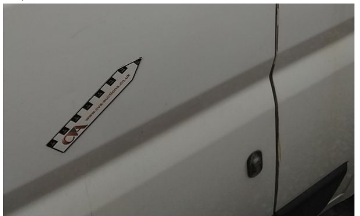
6: Door Moulding nsf Missing Replace
