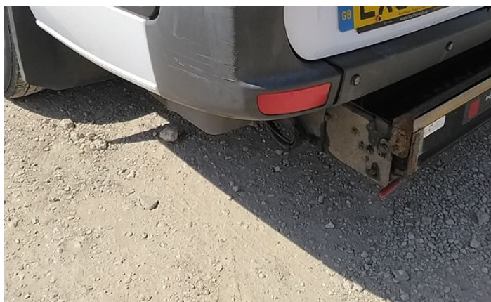
10: Qtr Panel Arch Extension ns Scuffed (Unpainted) Over 100mm
