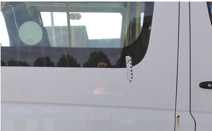
11: Qtr Panel osr Rusted Over 5mm
