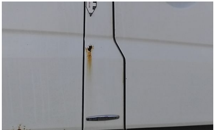
12: Qtr Panel osr Rusted Over 5mm
