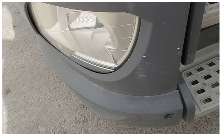
4: Bumper Front Grill Broken Replace
