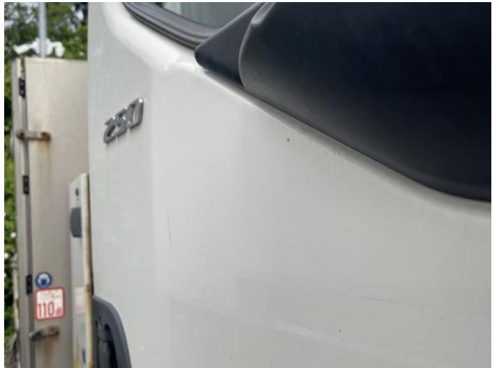
6: Door osf Dented Over 30mm
