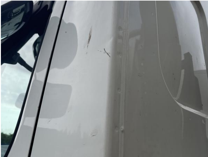
10: B Post ns Dented With Paint Damage
