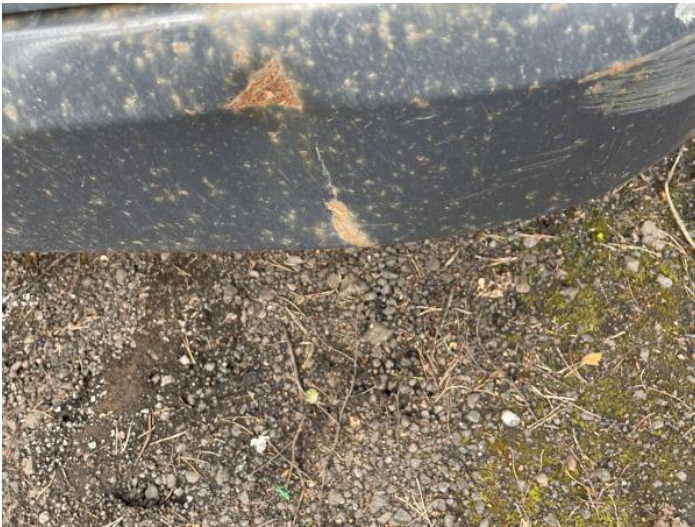
5: Bumper Front Rusted Over 5mm
