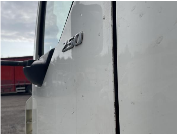
11: Door nsf Dented Over 30mm
