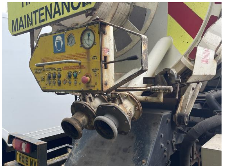
8: Tailgate Rusted Over 5mm
