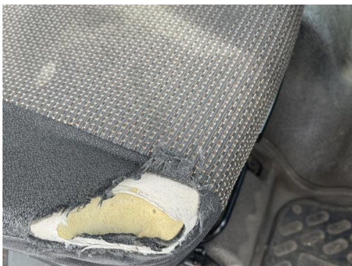
1: Seat Base Cover osf Torn Over 3mm
