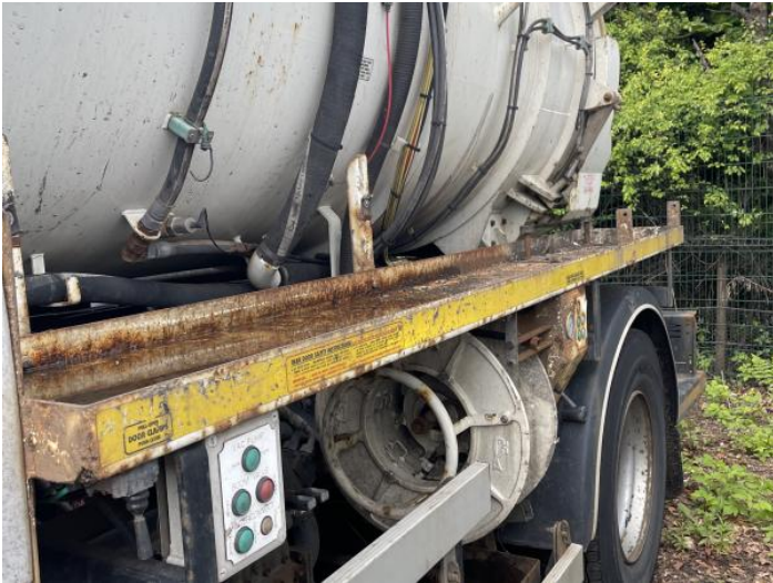
9: Qtr Panel nsr Rusted Over 5mm
