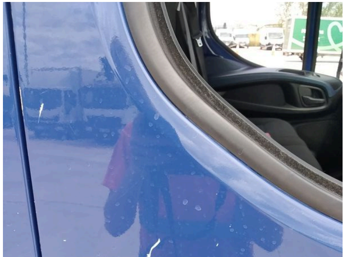
2: Door osf Scratched Over 25mm Thru Paint
