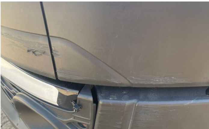
11: Wing nsf Dented With Paint Damage
