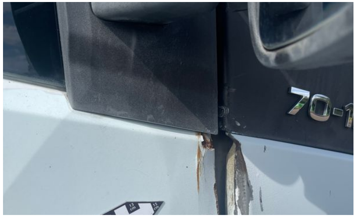
4: Wing Front Arch Extension os Scuffed (Unpainted) UpTo 100mm
