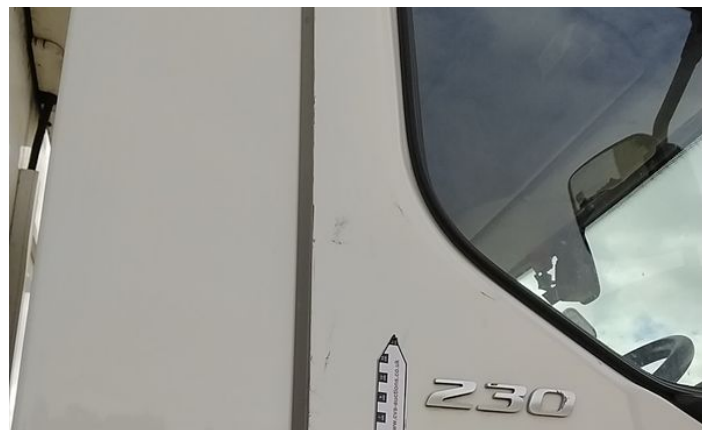
11: Door osf Scratched Over 25mm Not Thru Paint
