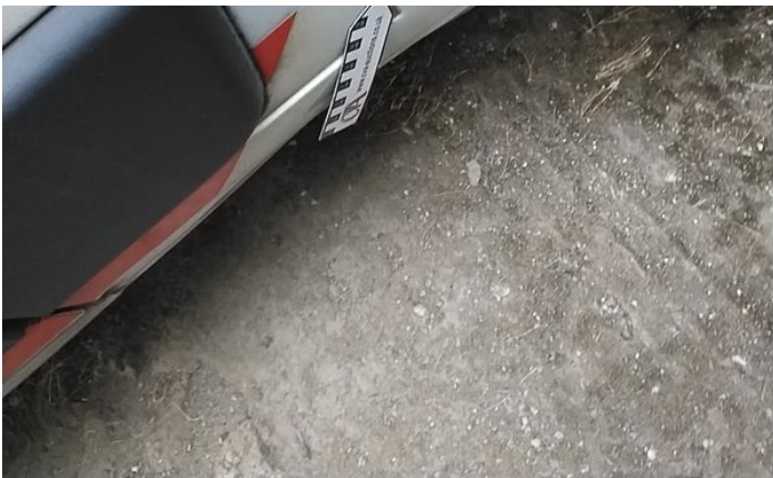
5: Qtr Panel nsr Dented Over 30mm
