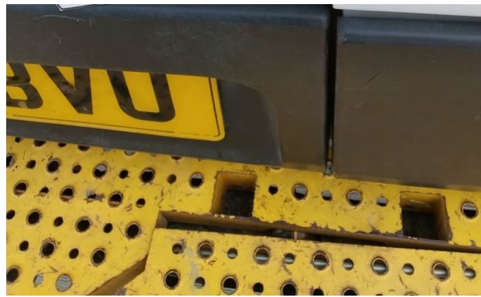
15: Door nsr Dented Over 30mm
