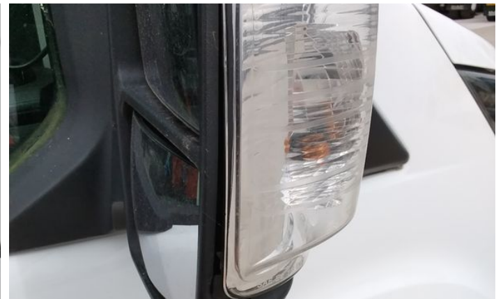
18: Lamp osr Broken Replace
