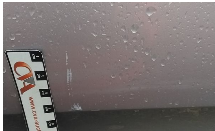
5: Door osr Dented With Paint Damage
