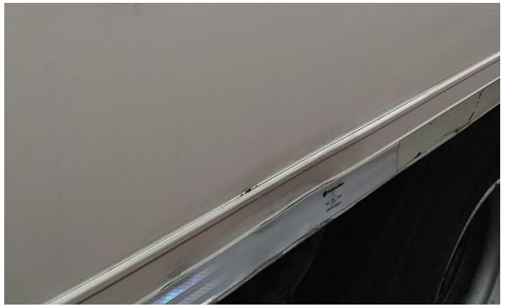
4: Door nsf Rusted Over 5mm
