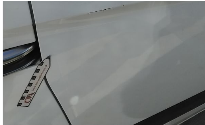
9: Door nsr Dented With Paint Damage
