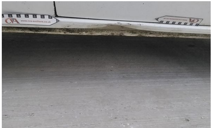
10: Door nsr Scratched Over 25mm Thru Paint
