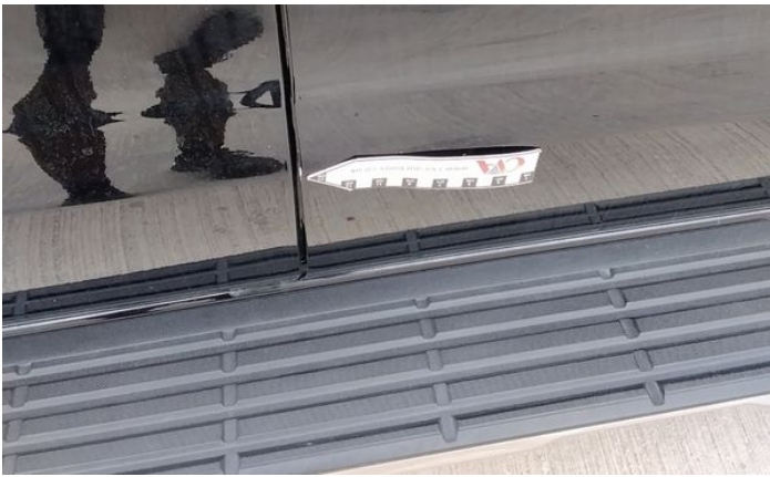
9: Qtr Panel osr Scratched Over 25mm Thru Paint
